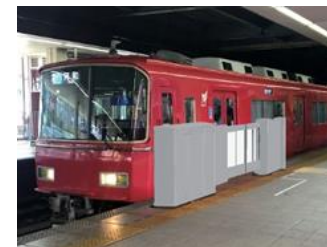
Pilot test for platform safety gates (Illustration)
