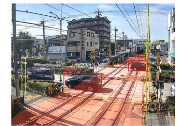
Physical detection of train crossing using an AI image analysis device (Illustration)
