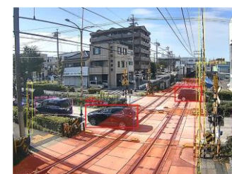
Physical detection of train crossing using an AI image analysis device (Illustration)
